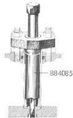
Fig. 8 Spreading of injector sleeve.
