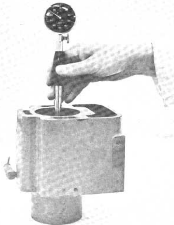
Fig. 17. Measuring cylinder bore wear
