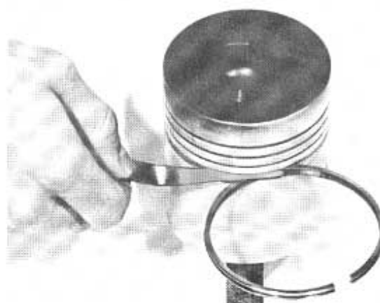
Fig. 18. Piston ring clearance in groove
